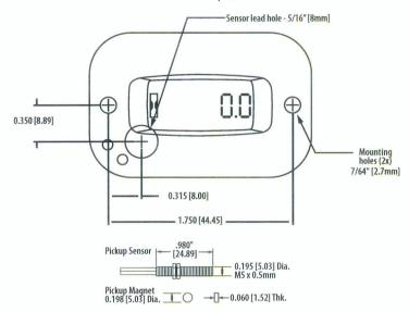
Included: GDI MotorTACH RPM pickup Sensor Motor shaft magnet disc
